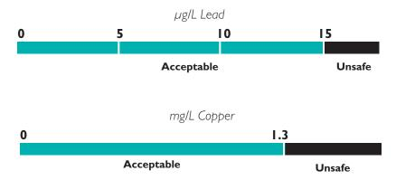
ACCEPTABLE RESULTS: less than 15  $\mu$ g/L (parts per billion) lead. Less than 1.3 mg/L (parts per million) copper
